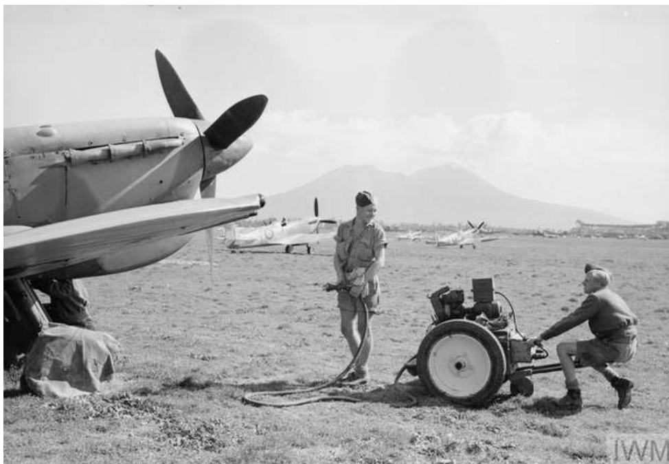
The ground crew prepares to start a Supermarine Spitfire Mark. VC of No. 324 Wing RAF at Capodichino near Naples, using a trolley accumulator. Spitfire Mark IXs of No. 93 Squadron RAF can be seen parked in the background, with Mount Vesuvius in the distance. IWM Catalogue No. CNA 4663.
